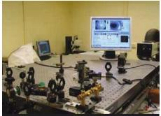
The adaptive optics system at the Visual Optics and Biophotonics laboratory, Spanish Council for Scientific Research (CSIC) is being used to gain a better understanding of basic mechanisms of the visual system
