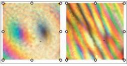
Singularity obtained in a white light beam passing a double-axial crystal placed between a matched polarizer and analyser, without a reference wave (left) and with a reference wave (right). After O V Angelsky *et al.* 2005 *Optics Express* **13(20)** 8179.
