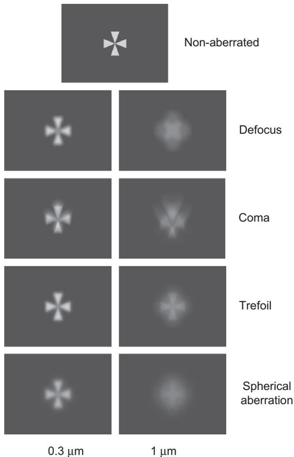
**Fig. 2.** Images of the nine targets used in this study. The non-aberrated Maltese cross is convolved with the PSF corresponding to 0.3 μm and 1 μm of defocus, vertical coma, vertical trefoil and spherical aberration (for a pupil of 3 mm).
