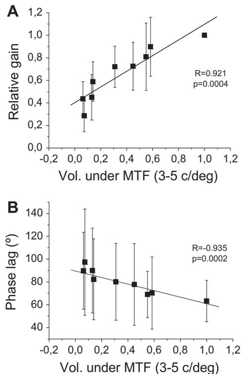
**Fig. 6.** Correlation between the relative gain (A) and the phase lag (B) averaged across subjects and the volume under the MTF between 3 and 5 c/deg.
