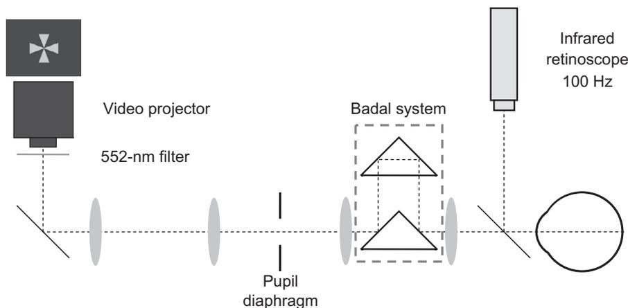
**Fig. 1.** Experimental set-up: the target is presented on the micro-mirror display of a video projector and its vergence (Zernike defocus) modified by means of a Badal optometer. Dynamic accommodation was recorded at 100 Hz with an infrared retinoscope.
