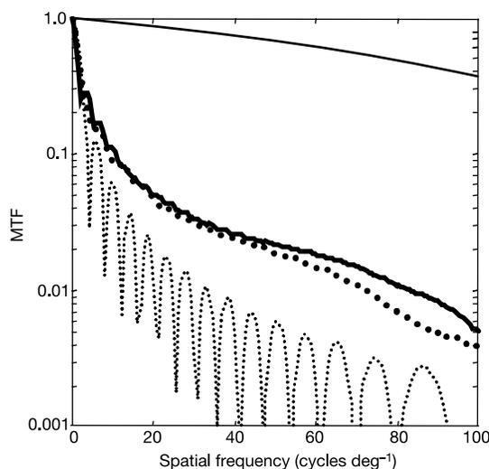
**Figure 1** MTFs at 550 nm (solid curves) and 450 nm (dotted curves) for two eyes: (1) a theoretical model eye subject to LCA but with no wave aberrations (thin lines) and (2) a real human subject's eye (thick lines). The other two subjects showed similar results. The
