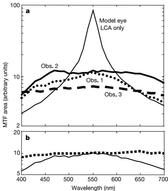
**Figure 2** MTF area. **a**, Area under the MTF (arbitrary units) as a function of wavelength for a theoretical model eye with LCA only and for three subjects with measured wave aberrations. **b**, Mean MTF area for all three subjects when defocus is set to optimize area at 550 nm (solid line) and when each wavelength is individually optimized (dashed line). The dashed line shows that MTF area at any single wavelength can be improved further by correcting focus at that wavelength.
