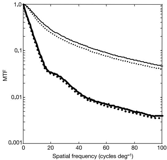
**Figure 4** Polychromatic MTFs for the theoretical model eye (thin lines) and for one subject (thick lines) with (solid lines) and without (dotted lines) the effect of macular pigment absorption at short wavelengths. Macular pigment produces only a trivial improvement in the MTF. The other two subjects showed similar results.
