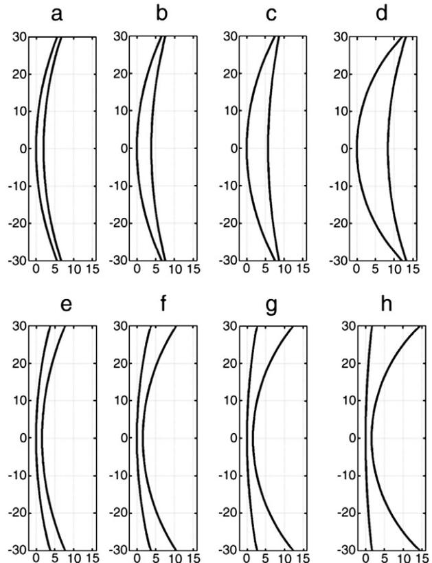
Fig. 3. Surface profiles of the lenses designed with the new procedure. Positive lenses: (a) 1 D (b) 3 D (c) 5 D (d) 7 D. Negative lenses: (e) -2.5 D (f) -5 D (g) -7.5 D (h) -10 D.
