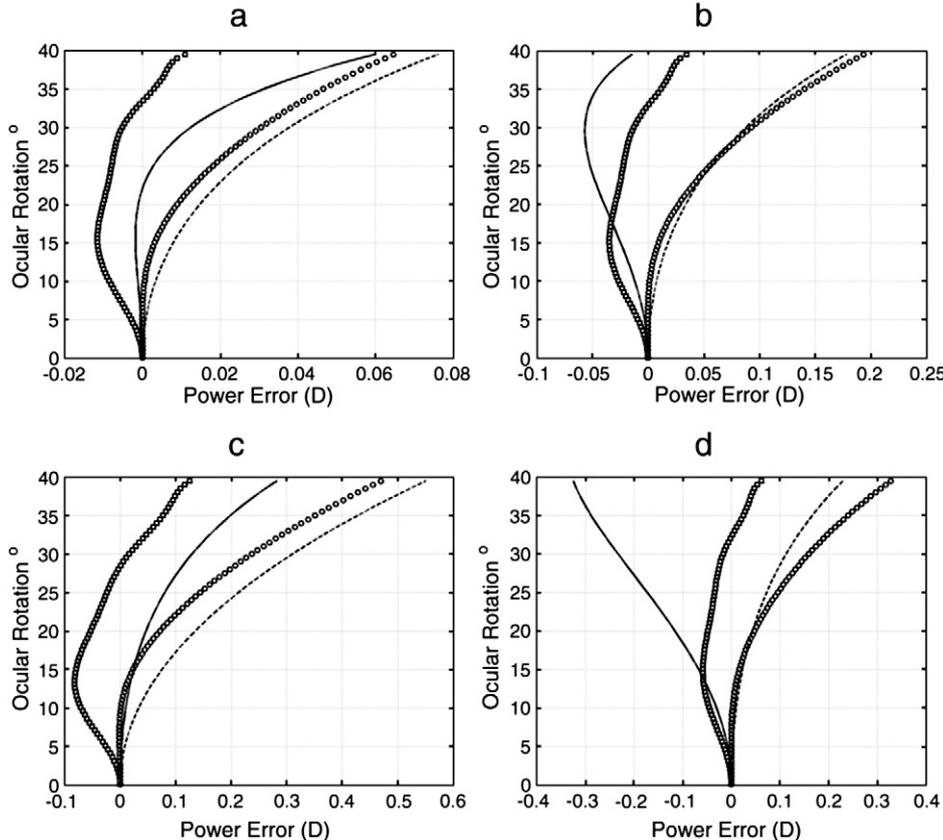
**Fig. 4.** Tangential and sagittal power error (D) as a function of ocular rotation (degrees) for the positive lenses: (a) 1 D (b) 3 D (c) 5 D (d) 7 D. Tangential and sagittal power error for the spherical lenses are plotted with solid and dashed lines respectively. Tangential and sagittal power error for the new aspheric lenses are plotted with squares and circles respectively.
