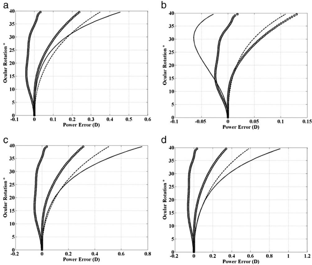
Fig. 5. Tangential and sagittal power error (D) as a function of ocular rotation (degrees) for the negative lenses: (a) –2.5 D (b) –5 D (c) –7.5 D (d) –10 D. Tangential and sagittal power error for the spherical lenses are plotted with solid and dashed lines respectively. Tangential and sagittal power error for the new aspheric lenses are plotted with squares and circles respectively.
