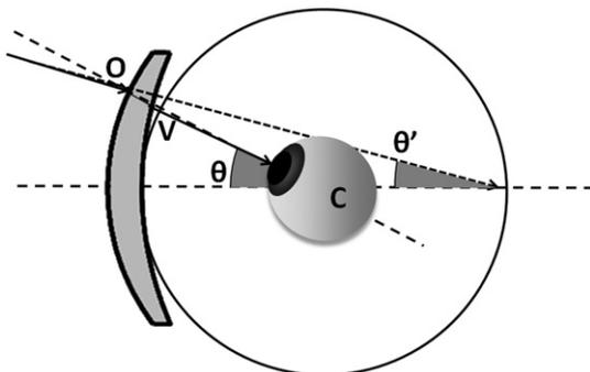
Fig. 1. General scheme to compute optical properties for different gaze directions. C is the center of rotation of the eye. V is the vertex sphere.
