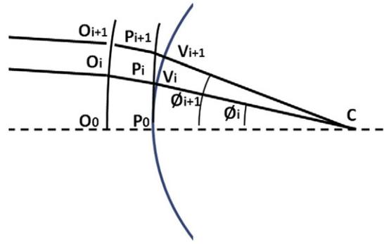
Fig. 2. Illustration of the design algorithm. C is the center of rotation of the eye.  $P_0$  and  $O_0$  are the back and front lens vertex points respectively.  $P_i$  and  $O_i$  denote points in the back and front lens surface respectively.  $V_i$  denote points  $i$  the vertex sphere.
