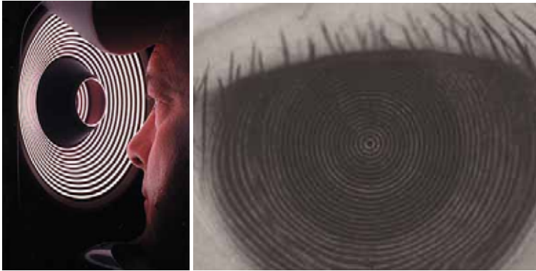
Fig. 2. 8. The Placido disks in a videokeratoscope (right side picture of Placido disks reflected on the anterior surface of a contact lens, from Kopf et al. (Kopf et al., 2008))
