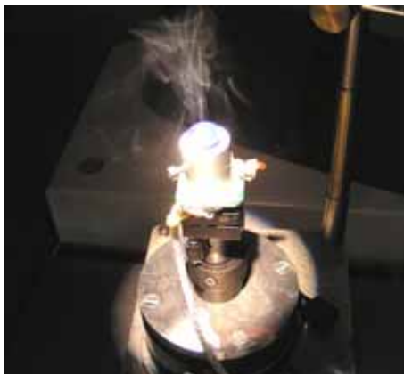
Fig. 5.8. Photograph of a flat artificial eye during the ablation with a clinical laser. Smoke and debris ejected from the ablation zone after repeated pulses could be shielding the following pulses. The exposure time was 1/3 seconds.
