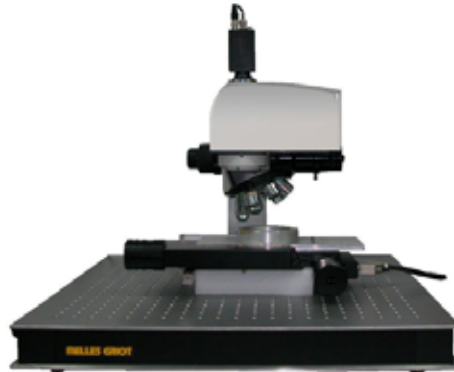
Fig. 2. 4. Non-contact confocal microscope used for profilometry measurements (PI \mu , Sensofar, Terrassa, Barcelona, Spain)
