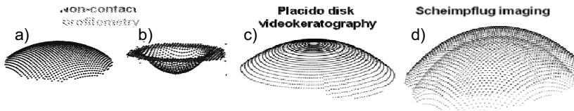
Fig. 2. 1. Examples of raw data obtained with the different instruments used to measure optical surfaces in this thesis. (a) Non-contact optical profilometry on spherical surfaces. (b) Non-contact optical profilometry on flat surfaces. (c) Atlas Videokeratography. (d) Pentacam Scheimpflug Imaging. Both the anterior and posterior surfaces of the cornea are measured.
