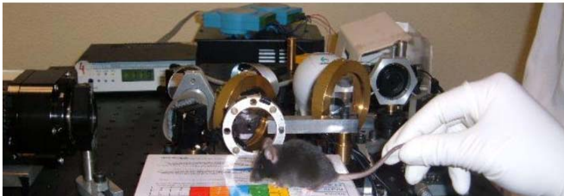
Figure 5.1. Mouse previous to measurements. Animal was placing in a platform in front of the Harman-Shack system near to IR ring LEDs.
