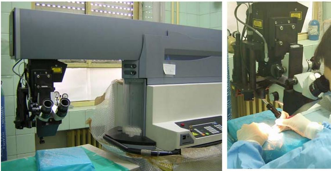
Figure 4.1. Photograph of the excimer laser (left) and a chick refractive surgery (right) used to perform surgery on chicks.
