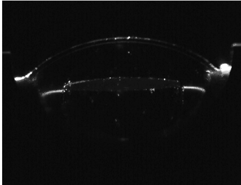
Figure 3.12. Scheimpflug image of an artificial eye of known dimensions (mm).
