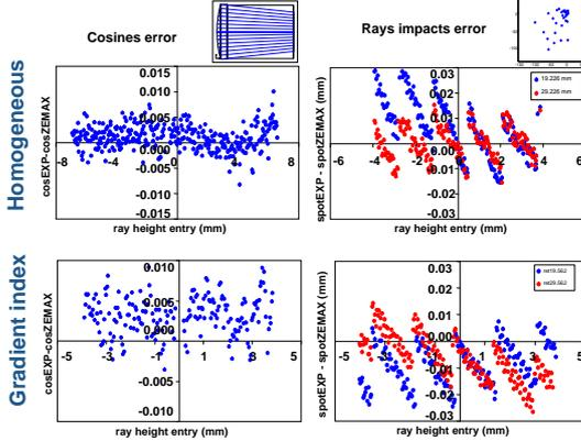
Average differences between the experimental and theoretical data are 0.005 in cosines (0.6 degrees) for lateral ray deflection and 20  $\mu\text{m}$  for ray aberration
