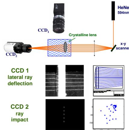
The x-y scanner combined with 150mm focal length lens delivers 200 rays to the lens with an estimated precision of  $11.5 \pm 0.8 \mu\text{m}$ .
