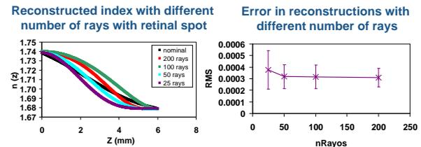
We found that, on average, GRIN is quite accurately reconstructed using less number of rays. Increasing the number of rays above 25 rays reduces variability.
