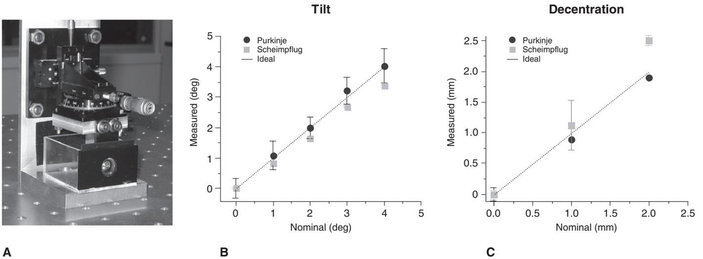
Figure 5. A. Photograph of the physical model eye used in the validations. B. Nominal versus estimated tilt. C. Nominal versus estimated decentration. ● represents data from Purkinje and ■ from Scheimpflug. Results are the average of three IOLs. The ideal X = Y line is also plotted.
