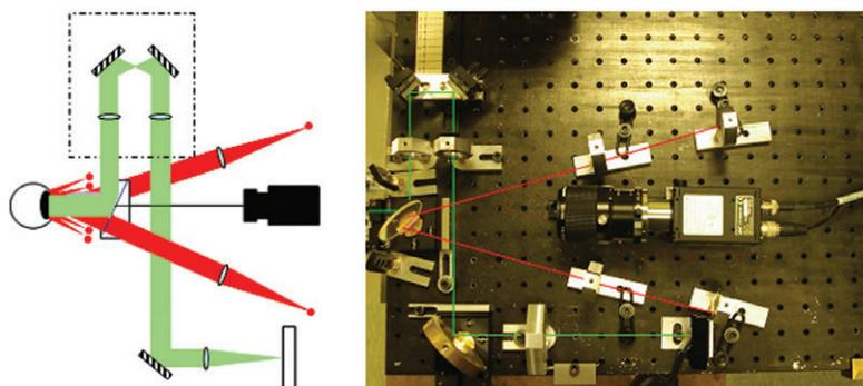
**Figure 1.** A Diagram of the Purkinje imaging system optical set-up. B. Photograph of the instrument at the Visual Optics and Biophotonics Lab, Instituto de Optica, CSIC.
