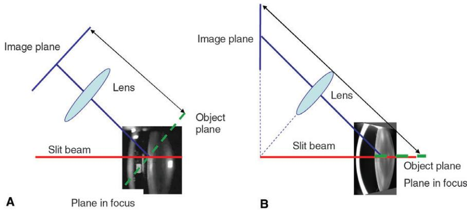
**Figure 3.** A. Principle of slitlamp imaging. A slit beam is focused on the eye and viewed with a microscope. The plane image and object image are parallel to each other. B. Principle of Scheimpflug imaging, where the image and objects planes are tilted with respect to each other in such a way that they intersect in one point.
