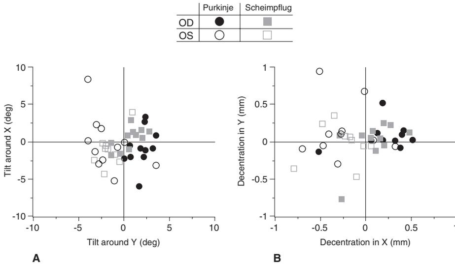
**Figure 7.** Tilt (A) and decentration (B) using Purkinje (●) and Scheimpflug (■) imaging. Solid symbols stand for right eyes and open symbols for left eyes. Refer to Figure 6 for sign conventions. The sign of the tilt around the X-axis has been changed to allow a more graphical representation of lens positioning, assuming a frontal view of the patients' eyes.
